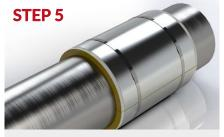
Cover the wrapped insulation foam with aluminum jacket.
